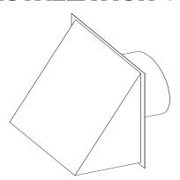
FIG. 15 Air Inlet Cap for Sidewall Termination
